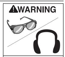
Operating this nailer can propel objects into the air, causing immediate eye damage. To protect yourself, always wear American National Standards Institute (ANSI) approved safety glasses or goggles when operating this equipment. In addition, this nailer discharges at 85-90 decibels. To protect your hearing, always wear ANSI approved ear protection when operating this nailer.
